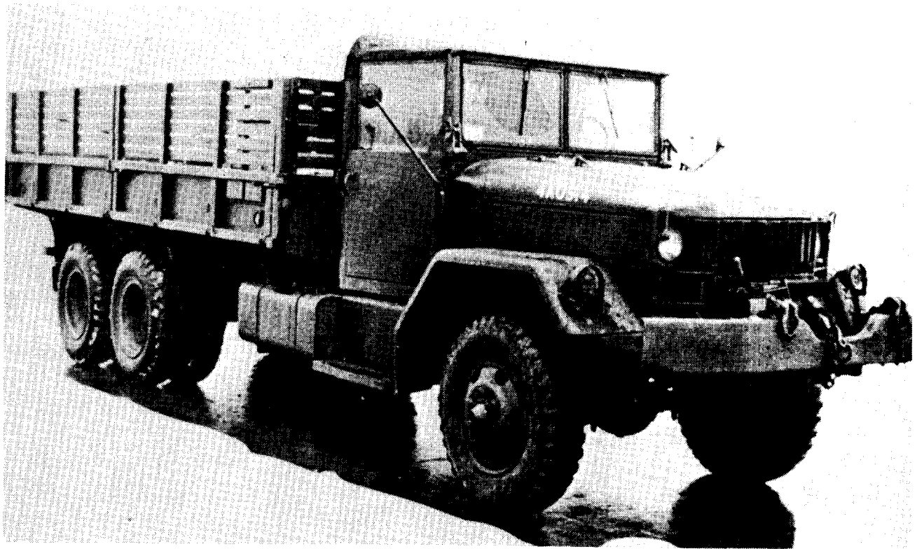
Figure 2-2. Truck, cargo, 2 1/2-ton, 6x6, M36
