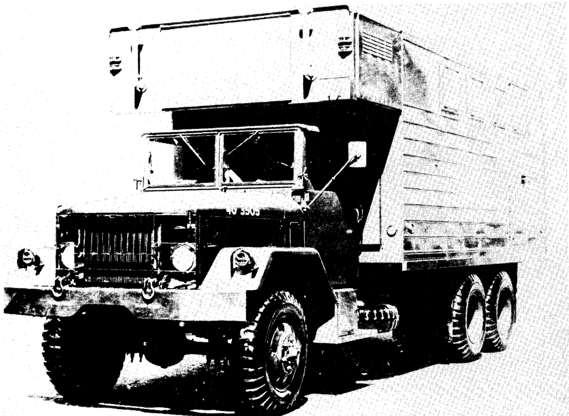
Figure 2-9. Truck, van, expandable, 2 1/2-ton, 6x6, M292.
